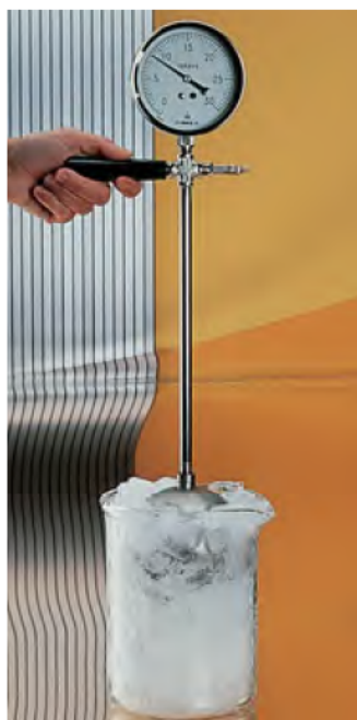
(a) A constant-volume gas thermometer
